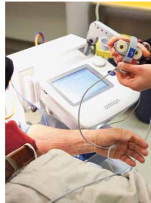
The new device measures and compares a patient's cardiovascular health and blood pressure via cuffs placed on their arms and legs.
